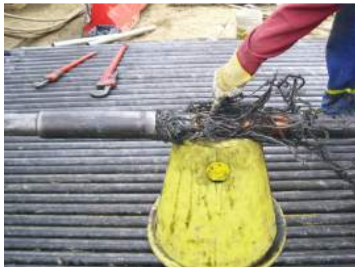
Braided line retrieves a stuck perforating gun
